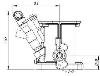
Bosch injector shown Remove spacer for Pico
